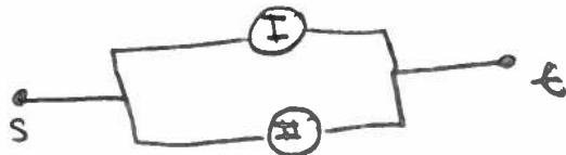
$$\begin{aligned} P(\text{electricity flows}) &= P(\text{I closes or II closes}) \\ &= P(\text{I closes}) + P(\text{II closes}) - P(\text{both}) \\ &= 0.9 + 0.9 - 0.9(0.9) = \underline{\underline{0.99}}. \end{aligned}$$
